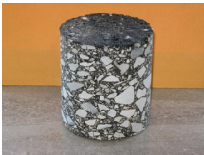
Figure 4-1. Test Specimen of asphalt concrete with mining waste (chat) making up part of the aggregate mix.
